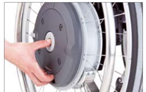
Removing the e-motion wheel from the wheelchair
